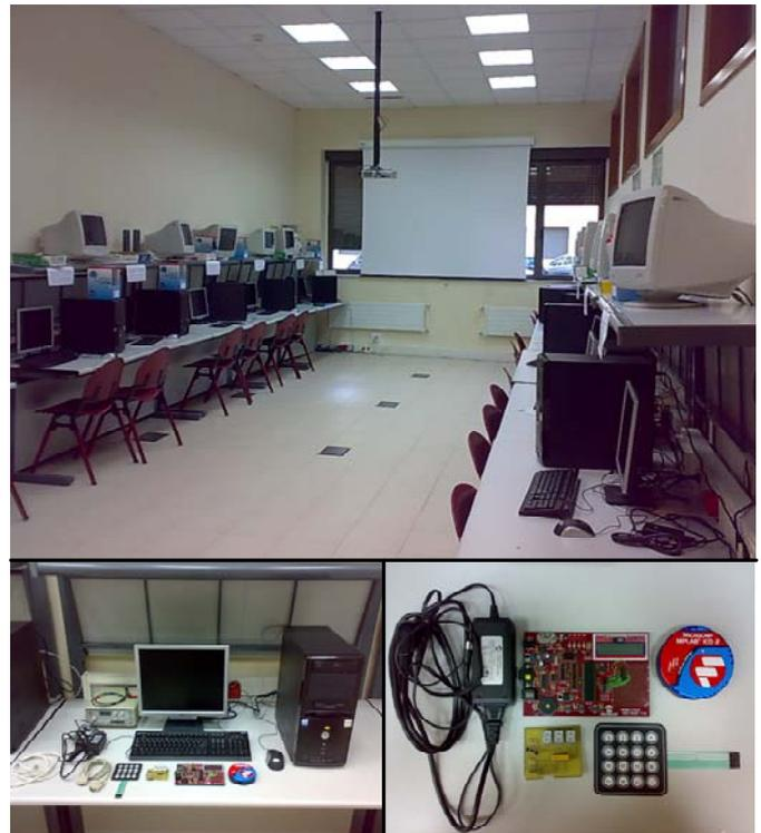
Figure 1. a) Laboratory with 12 workbenches for the practical classes; b) Workbench for every working group of 2-3 students; c) elements for debugging/testing the solution implemented for each project.
