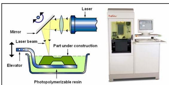
Figure 1. Stereolithography process and machine example.
