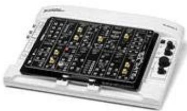
Fig. (1): Emona DATEX Set-up for Use in Communications Labs.
