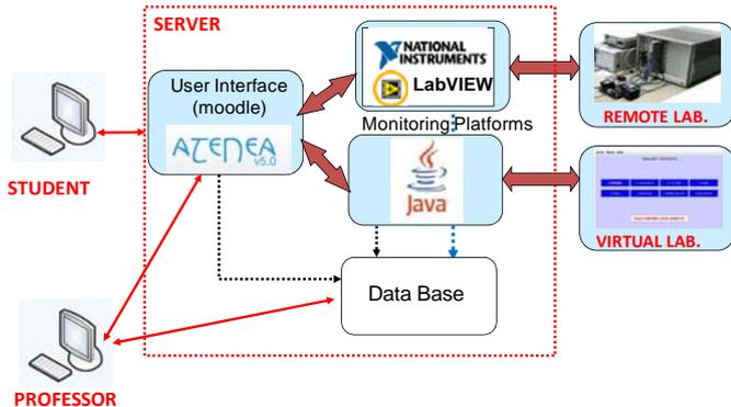
Figure 1. Remote laboratories and Virtual Laboratories are connected to the server through a software platform: Java or Labview. Atenea is the user interface (UPC Digital Campus).
