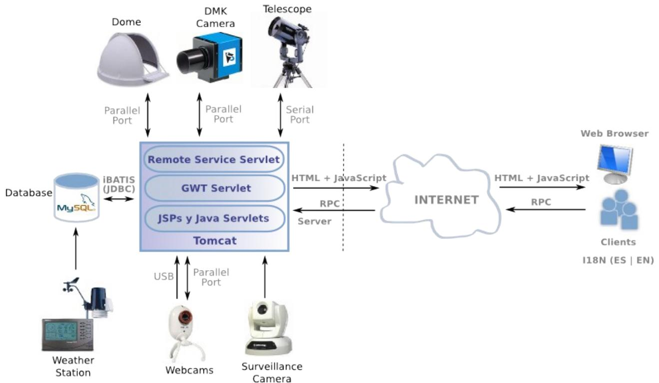
Figure 3. Montegancedo observatory's architecture
