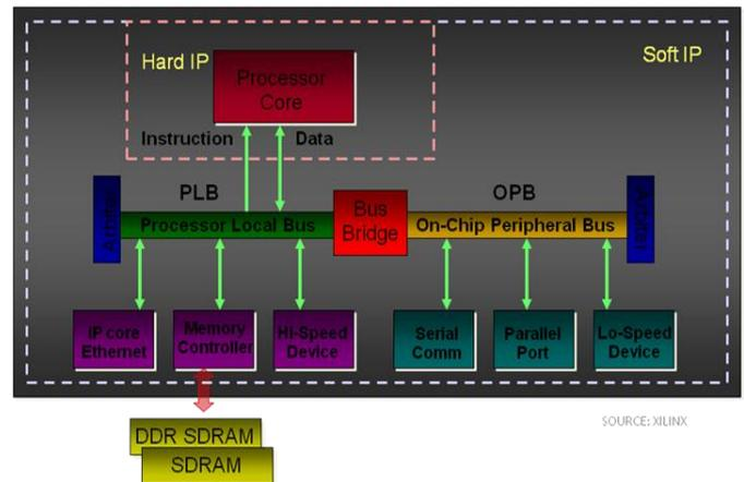
Figure 2. Xilinx embedded system hardware architecture [6]
