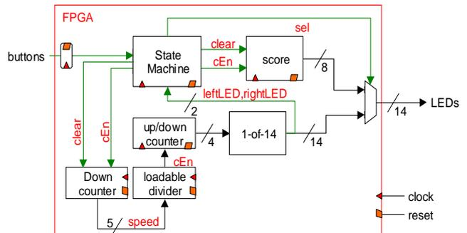
Figure 3. On-chip hardware setup for simple Game design
