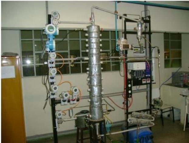
Figure 2. Pilot distillation column.
