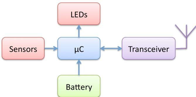
Figure 2. Block diagram of a basic WSN node.
