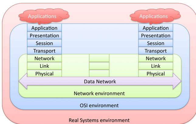
Figure 1. OSI reference model and associated environments.
