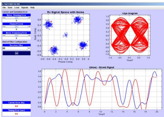
Figure 5. QAM LLS single step user window.
