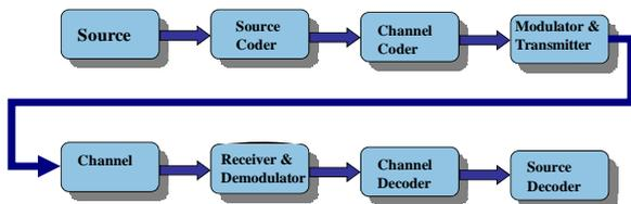
Figure 2. General Communication System functional diagram.
