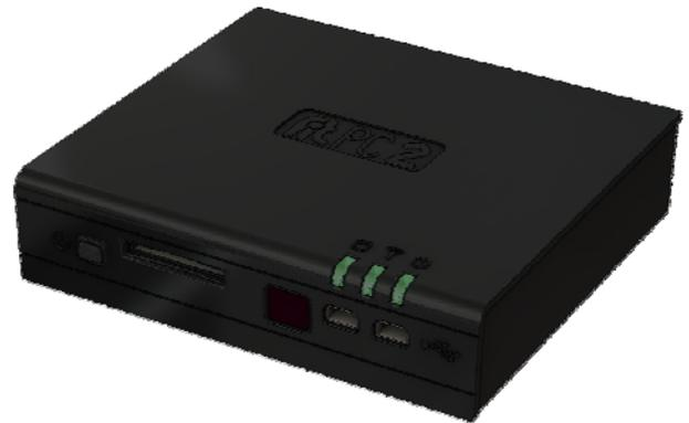
Figure 4. Low format computer “fit-pc2”
