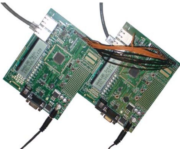
Figure 1. WebLab-DEUSTO-PIC v0.1 prototype
