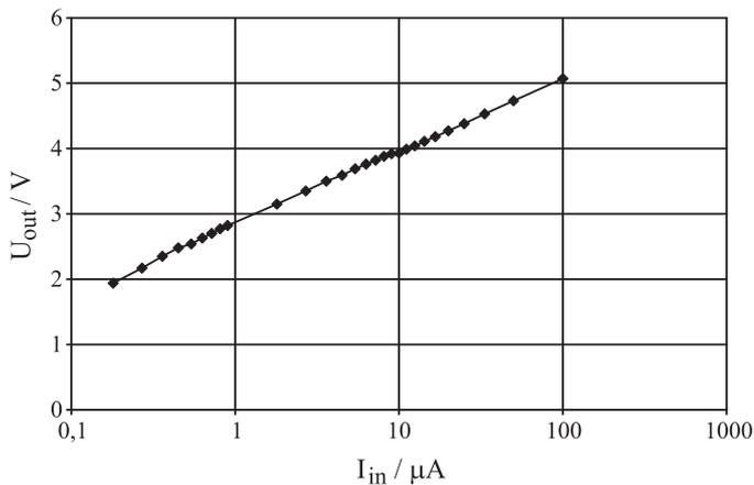
Figure 4. Response curve of logarithmic transimpedance amplifier
