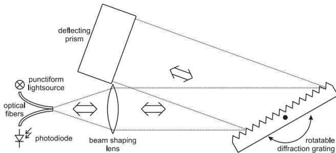
Figure 1. Optical setup of OSA
