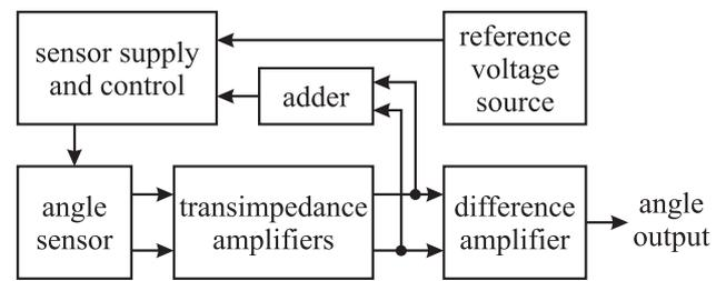
Figure 5. Block diagram of position sensor
