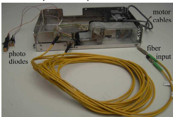
Figure 2. Opto-mechanical hardware of OSA
