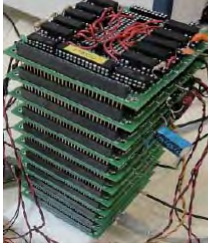
Fig. 2. VISIR Instruments and RSM boards assembly
