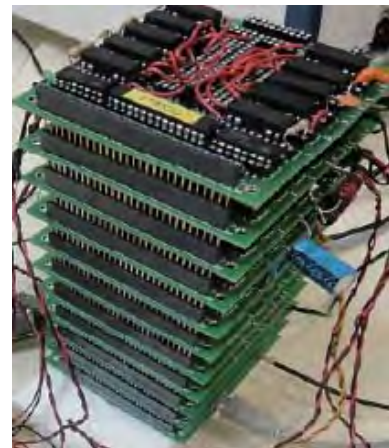
Figure 1. VISIR Instruments and RSM boards assembly
